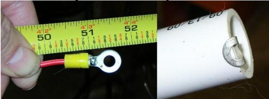
You can then tape the coax where it comes out of the PVC and drill holes for mounting Or for a bolt or cotter pin for setting the antenna on a smaller ,or in a larger support pipe. A EYE bolt can be added to hang the antenna from a rope(no metal wire) but you need to glue or use self tapping screws to give strength to the CAP. When hanging this and other antennas , you must give a rope support for the coax or it will be bad in a hurry. Also the coax can pull enough to damage your Big Stick .
