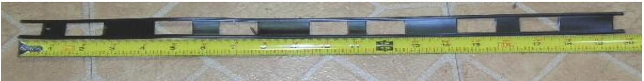
You then bare the lower legs to make the shunt feed and also bare the feed point at about 1" to 1 1/4" inches from the soldered shunt.
