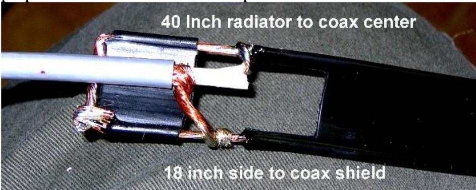
It should look like this, Note this was fed at just over 1 1/2" inches because it was for Air Band and not 2 Meters , but good enough photo of feed point. Yours should be about 1 1/4" inches from the bottom shunt.
