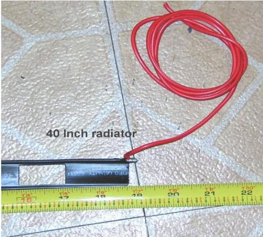
Once you have the SHUNT shunted and feed point bare , grab the PVC and slide the antenna end of your coax up through the PVC to the TOP of the antenna. Now is when you find out that at least 6 feet of coax is really needed. Bare the end of the coax and prepare it to connect to the feed point.
