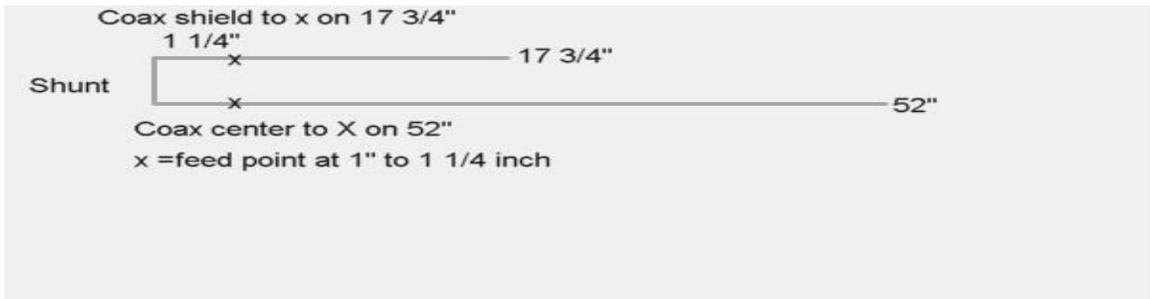
NOTE: To avoid confusion, The PVC Big Stick internal wire measures 52 inches on the side fed by the coax CENTER and the coax SHIELD feeds the 17 3/8" inch side. Some photos show wire lengths for a FREE HANGING (NO PVC) antenna.
