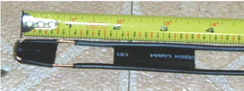
You then add about 35 inches of good wire , for the radiator ,to one side of the ladder line on the end away from the feed area . NOTE: The center of your coax connects to the LONGEST side (Total of 52 inches) and the shield connects to the 17 3/8" side.
