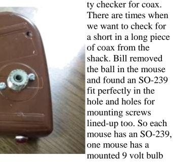
and battery inside. Bill even added a switch to turn the unit off and on. The idea is simple and the pro-ject cheap. Bill used the old hole where the cord was for the pilot light and filled the other hole and "wheel" slots with JB Weld. A coat of whatever paint was availa-ble finished off the project. Although an ohm meter would work as well, there are times when Bill's idea would be simpler and
